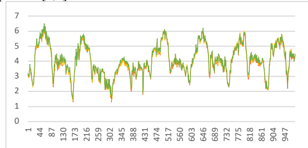
Fig. 7 – Monitored voltage total harmonic distortion (THD-U) for phases A, B, and C [%].
