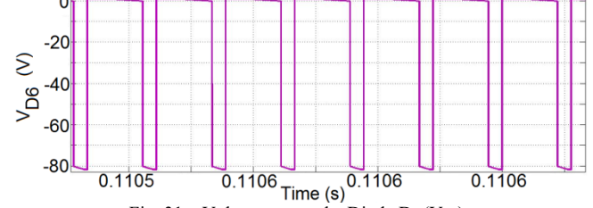
Fig. 31 – Voltage across the Diode D 6 ( V_{D6} )
