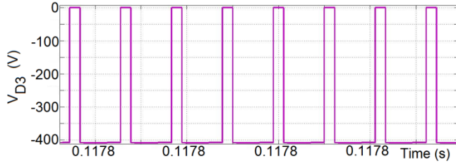
Fig. 25 – Voltage across the Diode D 3 ( V_{D3} )
