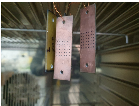
Fig. 6 – Contact samples aged in a forced air oven under a sodium chloride (NaCl) atmosphere [15,16].
