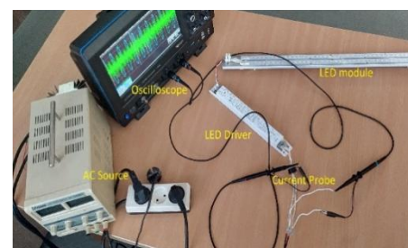
Fig. 4 – Test stand for measuring the conducted disturbance emission generated by the LED lamp under test in the frequency range 9 kHz-30 MHz.
