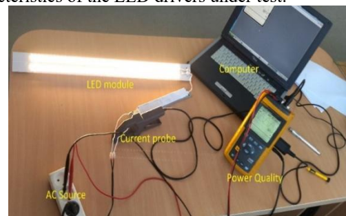
Fig. 3 – Test stand for measuring harmonic distortion generated by an AC/DC LED driver.
