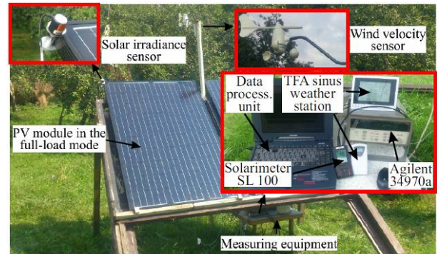
Fig. 2 – Photograph of the real experimental setup.
