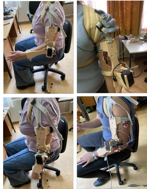
Fig. 3 – Photos of the orthosis attached to the shoulder girdle. The attached EMG electrodes are also visible in the right photos.
