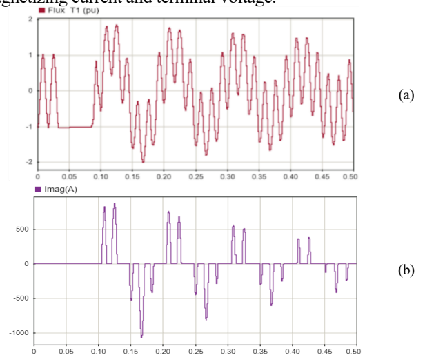
Fig. 6 –Impact of transformer saturation at a subsynchronous frequency:(a) Transformer core flux (b) Transformer magnetizing current.
