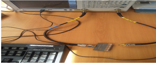
Fig. 13 – Testing of the four-element antenna array.
