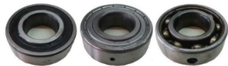
Fig. 6 – Ball bearing without and with holes on the outer race "holes of 3 mm and 6 mm diameters".
