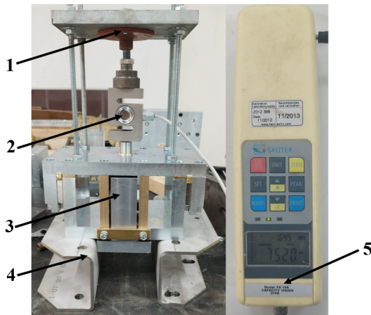
Fig. 19 – Measuring the holding force of the linear permanent magnet actuator (1 – variable spacing support, 2 – load cell sensor, 3 – linear actuator, 4- stainless steel support, 5 – digital force gauge).
