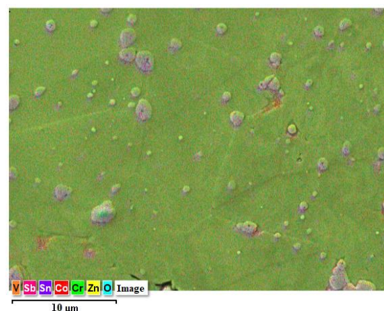
Fig. 10 – EDS layered image (5000 ×) of MOVs.
