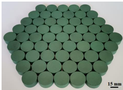
Fig. 7 – Macrograph image of the developed ZnO-V 2 O 5 -based varistors.
