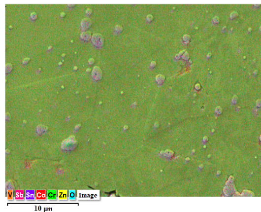
Fig. 10 – EDS layered image (5000 ×) of MOVs.
