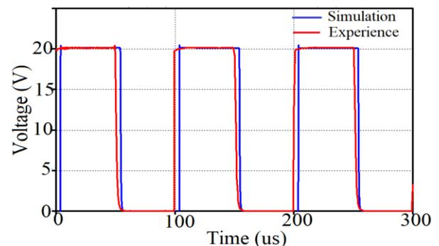
Fig. 6 – Temporal voltage response at the output of the series chopper.
