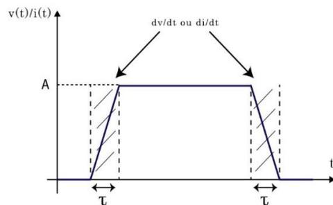
Fig. 1 – Trapezoidal waveform associated with switching [13].
