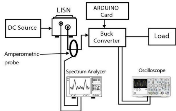
Fig. 5 – Descriptive diagram of the bench for measuring electromagnetic interference.
