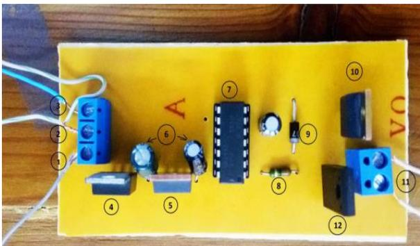
Fig. 3 – Printed circuit board of series chopper.
