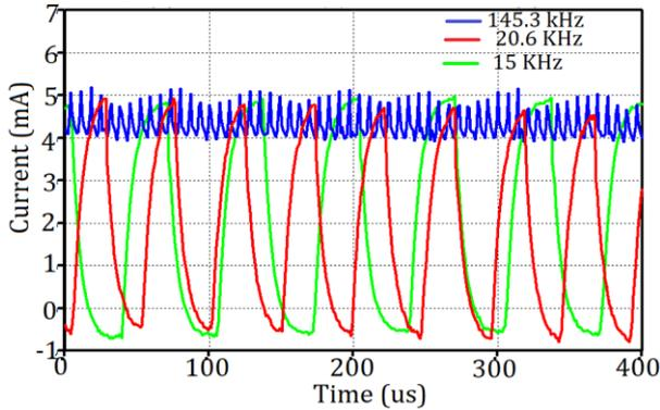
Fig. 13 – Temporal response of the input current as a function of the variation of the frequency of the MOSFET control signal generated by Arduino for duty cycle 50 %.
