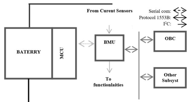
Fig.3 – BMS Hardware Architecture proposed.
