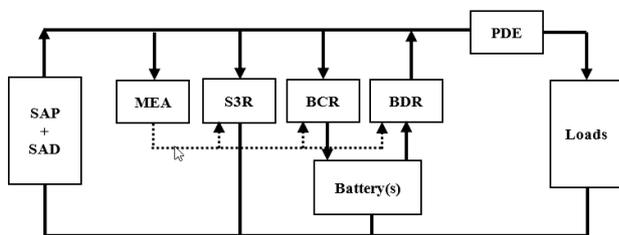
Fig. 1 – Regulated BUS Architecture.
