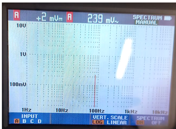
Fig. 9 – Frequency response of the piezoelectric cantilever.
