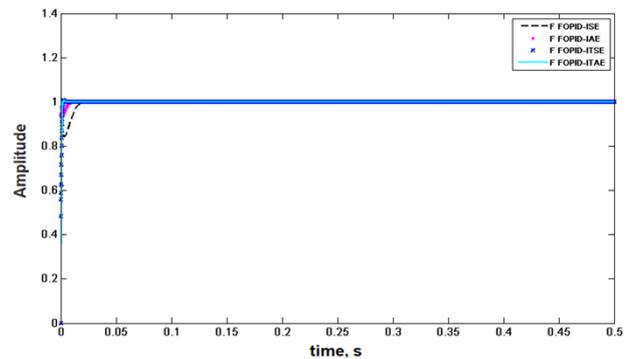
Fig. 10 – Step responses of IH system with fuzzy FOPID controller.
