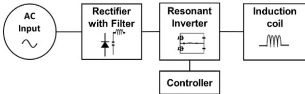
Fig. 1 – Typical induction heating system.
