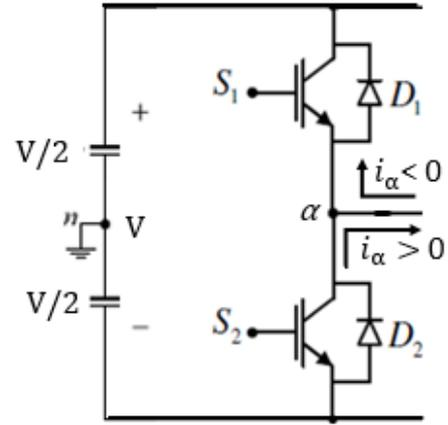
Fig. 4 – Typical VSI leg configuration.
