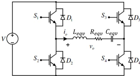
Fig. 2 – IH system having full-bridge resonant inverter.
