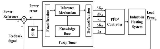
Fig. 7 – Representation of adaptive fuzzy FOPID controller.
