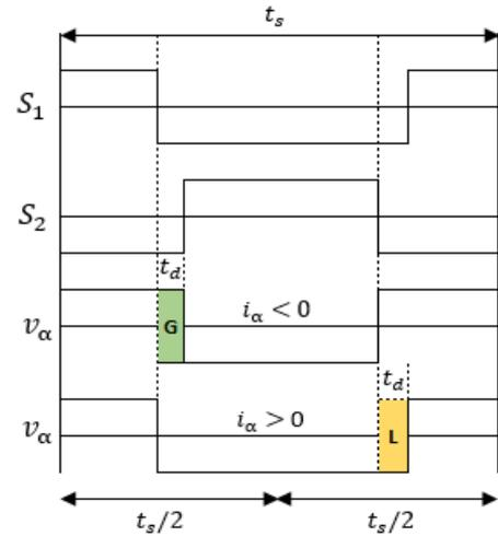
Fig. 5 – Switching patterns and output voltages including dead-time effect.
