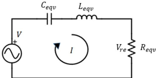
Fig. 3 – Simplified inverter circuit.
