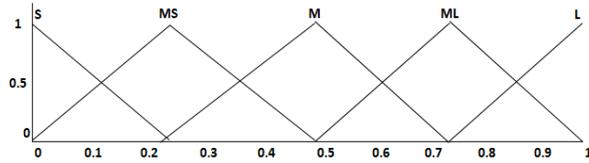
Fig. 8c – Membership functions for  $\Delta K_p$ ,  $\Delta K_i$ ,  $\Delta K_d$ ,  $\Delta \lambda$ ,  $\Delta \mu$ .
