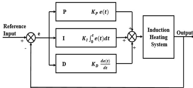
Fig. 6 – Representation of IOPID controller.
