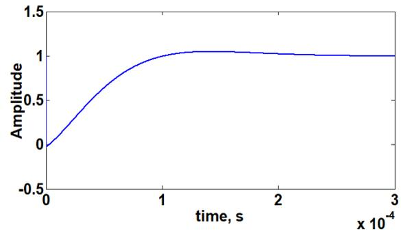
Fig. 9 – Step response of IH system having IOPID controller.
