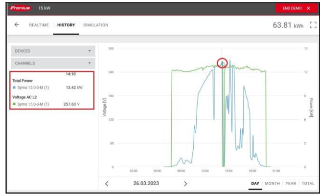
Fig. 10 – Overvoltage of the low voltage grid.
