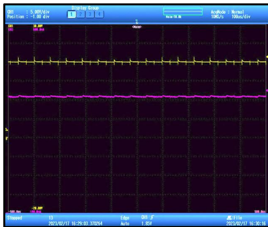
Fig. 15 – LED current waveform of resonant SEPIC with Vfc LED driver.
