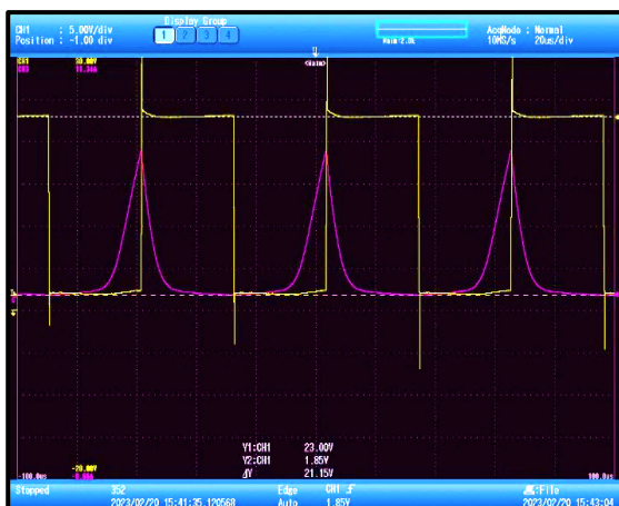
Fig. 16 – Voltage and current stress across the switch in resonant SEPIC with Vfc LED driver.
