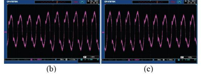
Fig. 5 – Load current i_L : a) load current waveform; b) i_L during load increasing; c) i_L during load decreasing.
