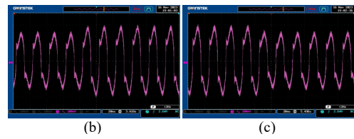
Fig. 5 – Load current i_L : (a) Load current waveform (b) i_L during load increasing (c) i_L during load decreasing.
