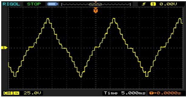
Fig. 8 – Hardware result of 13-level MLI.
