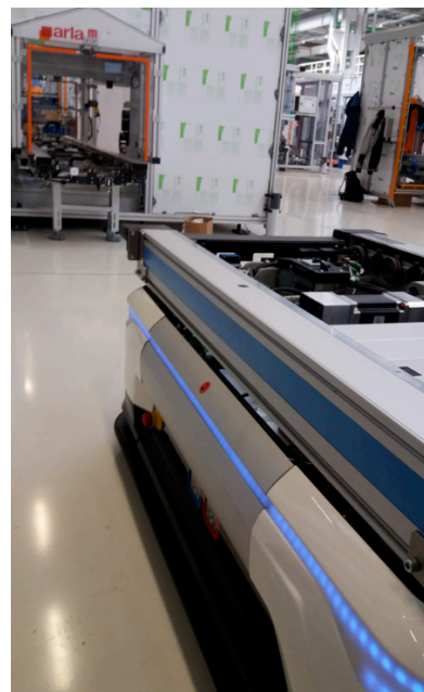
Fig. 2 – The AGV collecting a test piece from the current station.
