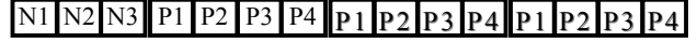
Fig. 3 – Structure of a chromosome to represent a possible solution of the LDVS optimization problem.
