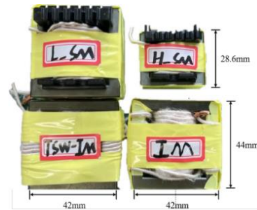
Fig. 15 – Comparison of magnetic parts.
