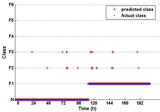
Fig. 9 – SVM diagnosis test result: short-circuit one cell (F1).
