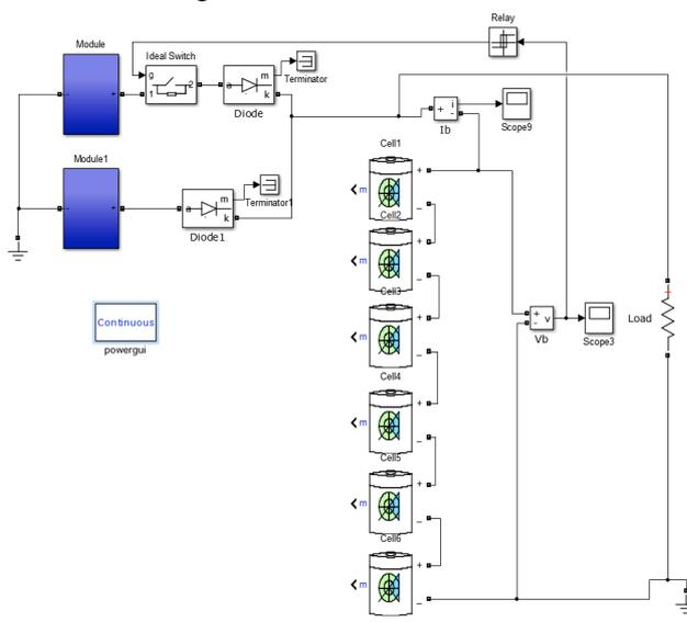
Fig. 1 – SimPowerSystem implementation of SAPV system.
