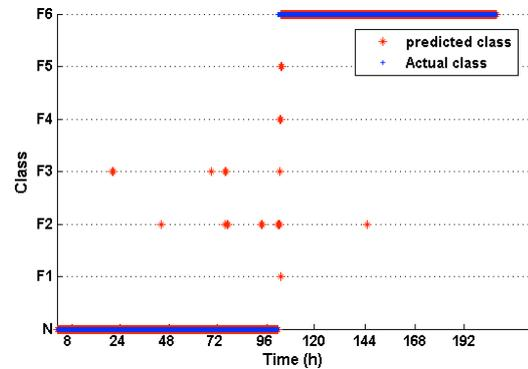
Fig. 13 – SVM diagnosis test result: short-circuit six cells (F6).
