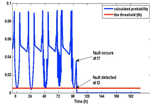
Fig. 12 – Anomaly detection test result: short-circuit six cells (F6).
