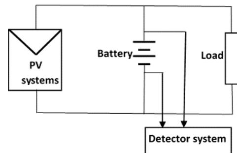
Fig. 2 – Schematic block of detector system used in Battery for SAPV system.
