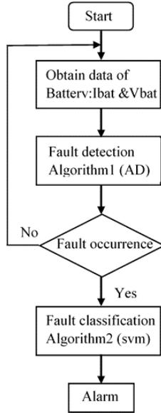
Fig. 3 – Flowchart of the proposed fault diagnosis process.
