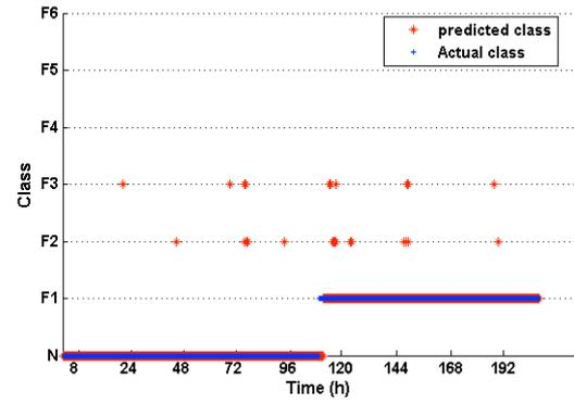
Fig. 11 – SVM diagnosis test result: short-circuit three cells (F3).
