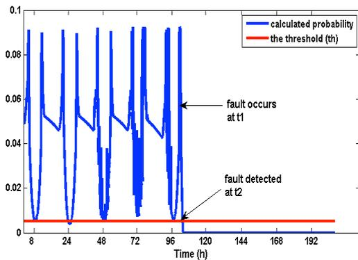
Fig. 10 – Anomaly detection test result: short-circuit three cells (F3).
