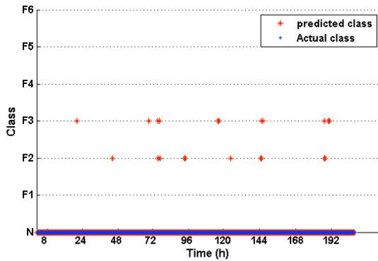
Fig. 7 – SVM diagnosis test result: normal case.
