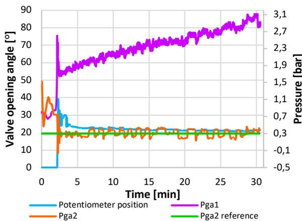
Fig. 9 – Valve experimental data acquired with PID control.
