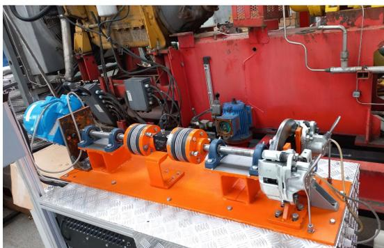
Fig. 2 – Valve test bench with brake.
