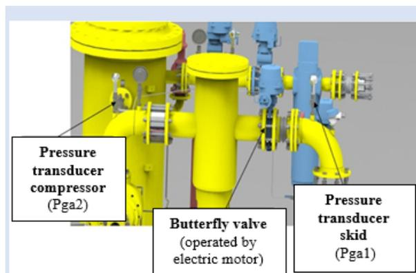
Fig. 6 – Valve installed on screw compressor skid.
