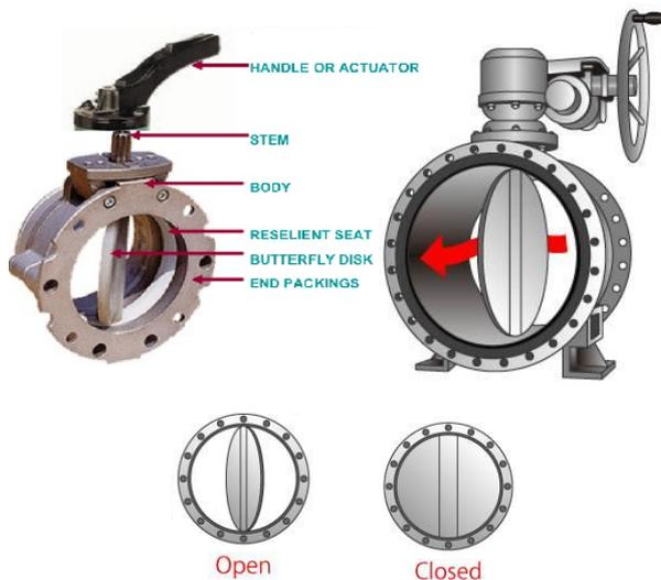
Fig. 1 – Butterfly valve construction and working principle [16].
