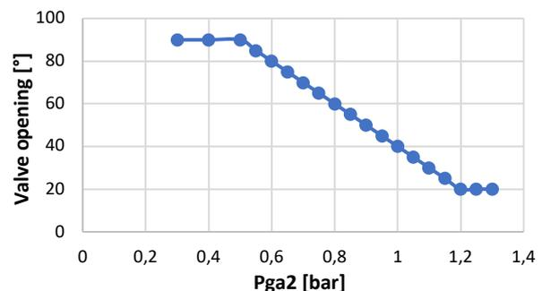
Fig. 10 – SDV opening with respect to the pressure in the compressor.
