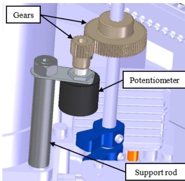
Fig. 7 – 3D model showing the potentiometer mounted for providing valve position feedback.
