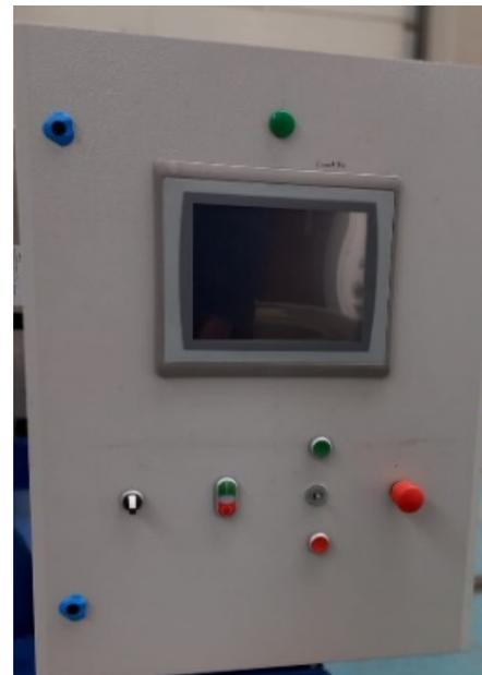
Fig. 4 – Control cabinet front door.
