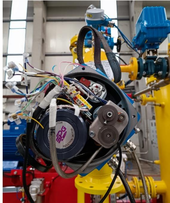
Fig. 3 – Valve installed on screw compressor skid.
