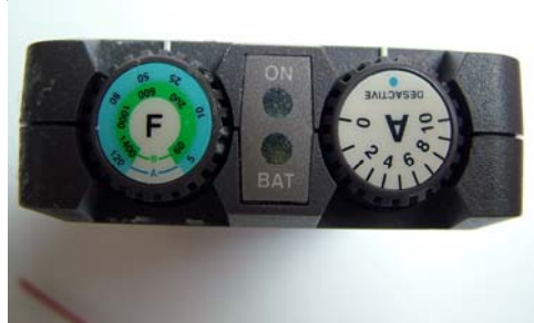
Fig. 2 – The control panel of the Interstim Neurostimulator
