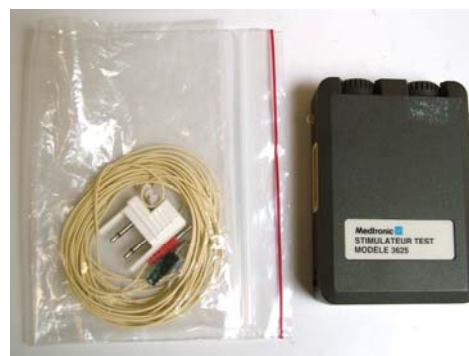
Fig. 3 – Test stimulation using long term lead.
