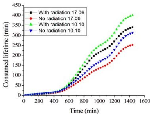
Fig. 13 – Time variation of the consumed lifetime for T1 on 17.06.2019 (black/red curves) and on 10.10.2019 (green/blue curves), both in the presence (black/green curves) and in the absence of the solar radiation (red/blue curves),  $\theta_h$  – calculated with FDM.
