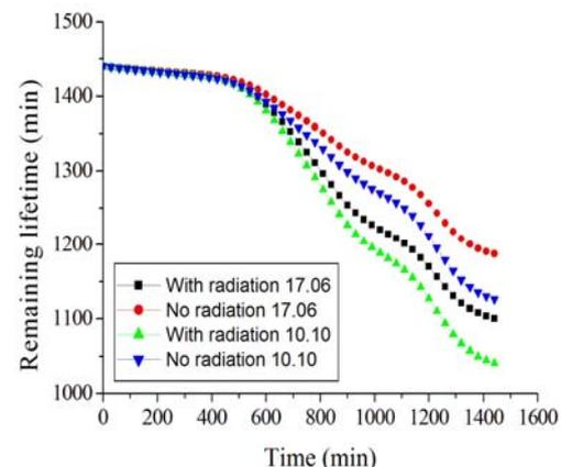
Fig. 16 – Time variation of the remaining lifetime for T1 on 17.06.2019 (black/red curves) and on 10.10.2019 (green/blue curves), both in the presence (black/green curves) and in the absence of the solar radiation (red/blue curves) ( $\theta_h$  – calculated with FDM).
