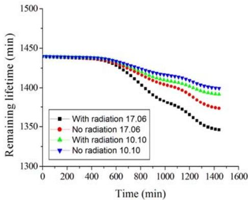
Fig. 17 – Time variation of the remaining lifetime for T2 on 17.06.2019 (black/red curves) and on 10.10.2019 (green/blue curves), both in the presence (black/green curves) and in the absence of the solar radiation (red/blue curves) ( $\theta_h$  – calculated with FDM).
