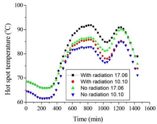
Fig. 6 – Time variation of the hot spot temperature for T2, on 17.06.2019 (black/green curves) and on 10.10.2019 (red/blue curves), both in the absence (green/blue curves) and in the presence of solar radiation (black/red curves) calculated with M2 method.
