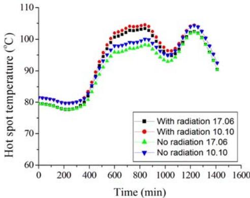
Fig. 4 – Time variation of the hot spot temperature for T1 on 17.06.2019 (black/green curves) and on 10.10.2019 (red/blue curves), both in the absence (green/blue curves) and in the presence of solar radiation (black/red curves) calculated with M2 method.
