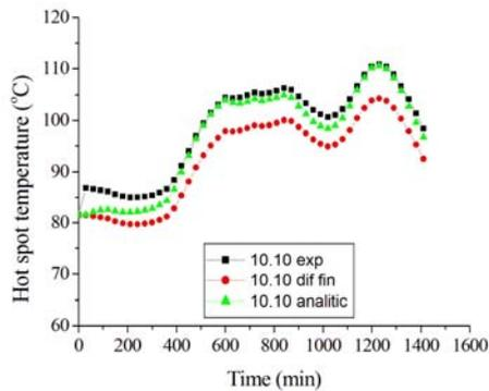
Fig. 9 – Time variation of the hot spot temperature for T1 on 10.10.2019, calculated using exponential functions method (black curve), analytical method (green curve) and finite differences method (red curve) (in the absence of the solar radiation).
