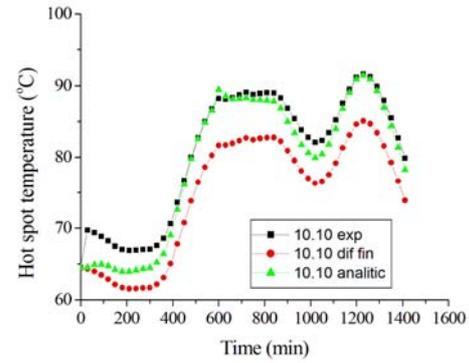
Fig. 11 – Time variation of the hot spot temperature for T2 on 10.10.2019, calculated using exponential functions method (black curve), analytical method (green curve) and finite differences method (red curve) (in the absence of the solar radiation).
