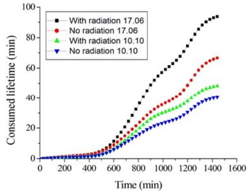
Fig. 14 – Time variation of the consumed lifetime for T2 on 17.06.2019 (black/red curves) and on 10.10.2019 (green/blue curves), both in the presence (black/green curves) and in the absence of the solar radiation (red/blue curves),  $\theta_h$  – calculated with FDM.
