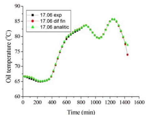
Fig. 12 – Time variation of the oil temperature for T1 ( $P_s = 0$ ), calculated with EFM (black curve), FDM (red curve) and AM (green curve).
