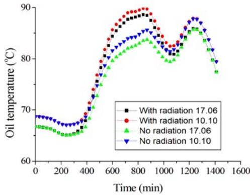
Fig. 3 – Time variation of the oil temperature for T1 on 17.06.2019 (black/green curves) and on 10.10.2019 (red/blue curves), both in the absence (green/blue curves) and in the presence of solar radiation (black/red curves).
