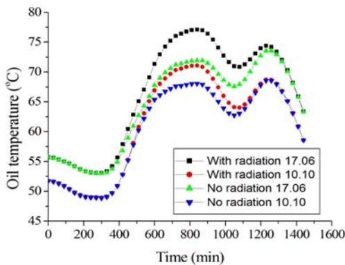
Fig. 5 – Time variation of the oil temperature for T2 on 17.06.2019 (black/green curves) and on 10.10.2019 (red/blue curves), both in the absence (green/blue curves) and in the presence of solar radiation (black/red curves) calculated with M2 method.
