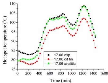
Fig. 8 – Time variation of the hot spot temperature for T1 on 17.06.2019, calculated using exponential functions method (black curve), analytical method (green curve) and finite differences method (red curve) (in the absence of the solar radiation).
