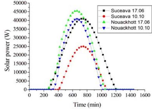
Fig. 2 – Time variation of solar power in Nouakchott (green/blue curves) and Suceava (black/red curves), on 17.06.2019 (green/black curves) and on 10.10.2019 (red/blue curves).
