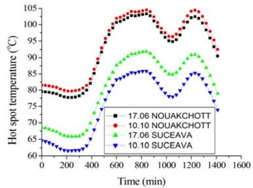
Fig. 7 – Time variation of the hot spot temperature in the presence of solar radiation for T1 (black/red curves) and T2 (green/blue curves), on 17.06.2019 (black/green curves) and on 10.10.2019 (red/blue curves) (obtained using finite differences method) calculated with M2 method.
