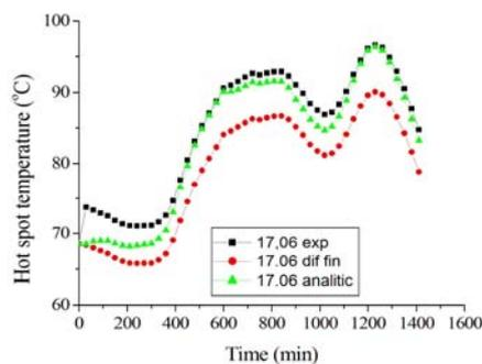
Fig. 10 – Time variation of the hot spot temperature for T2 on 17.06.2019, calculated using exponential functions method (black curve), analytical method (green curve) and finite differences method (red curve) (in the absence of the solar radiation).
