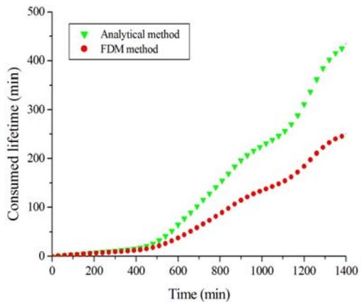
Fig. 15 – Time variation of the consumed lifetime for T2 on 17.06.2019 in the absence of the solar radiation, calculated with FDM (green curve) and analytical method (red curve).
