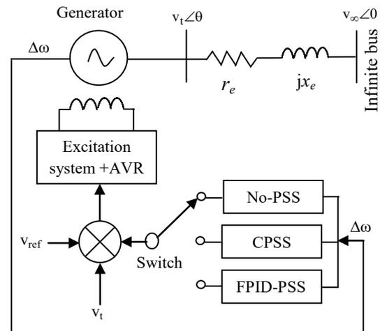
Fig. 1 – SMIB system the excitation of the generator.
