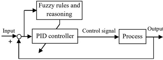
Fig. 4 – PID control system with a fuzzy gain scheduler.
