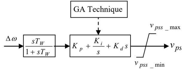
Fig. 3 – Structure of PID type PSS.
