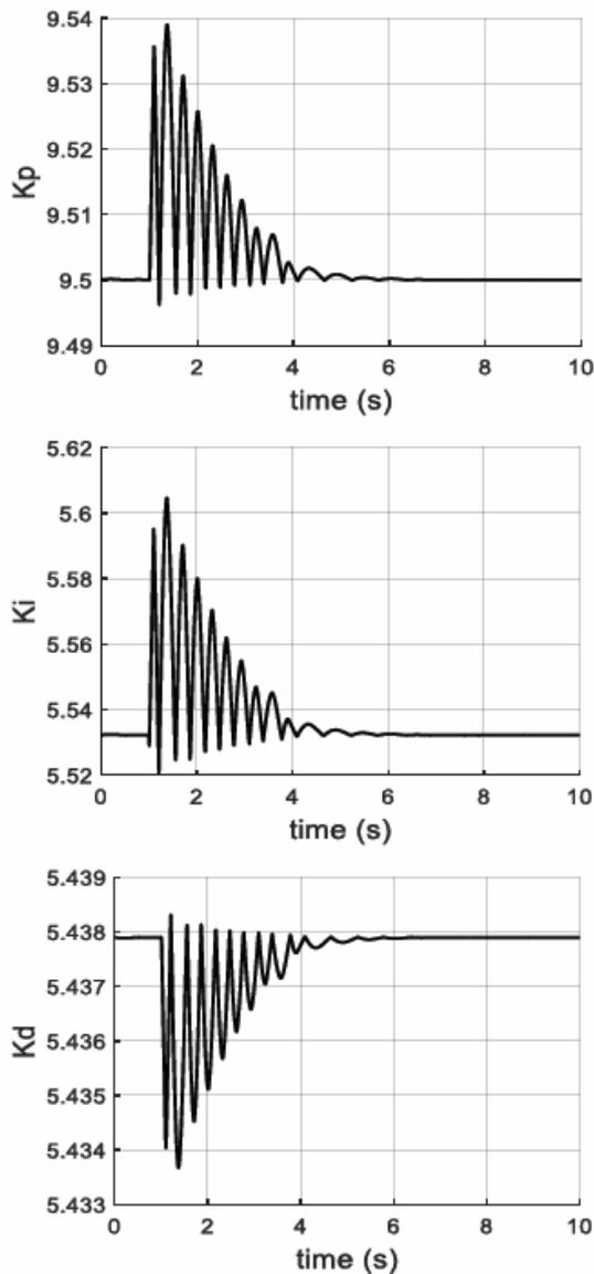
Fig. 8 – PID parameters of the fuzzy gain scheduler for the control of the system.
