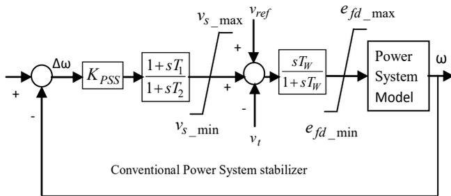
Fig. 2 – Block diagram of the PSS and the excitation system.
