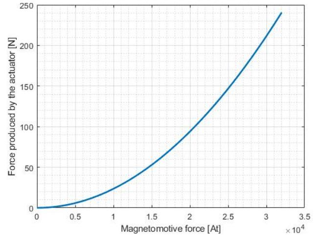
Fig. 5 – Relation between mechanical force and magnetomotive force.
