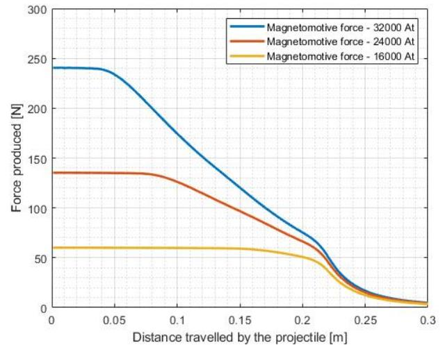
Fig. 6 – Relation between mechanical force and distance, for different magnetomotive forces.
