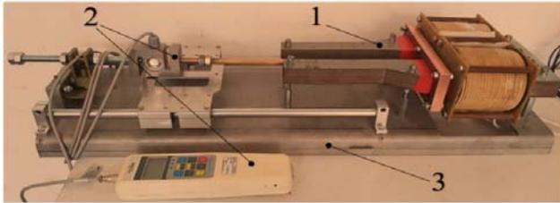
Fig. 10 – Physical model of the alternative current actuator.
