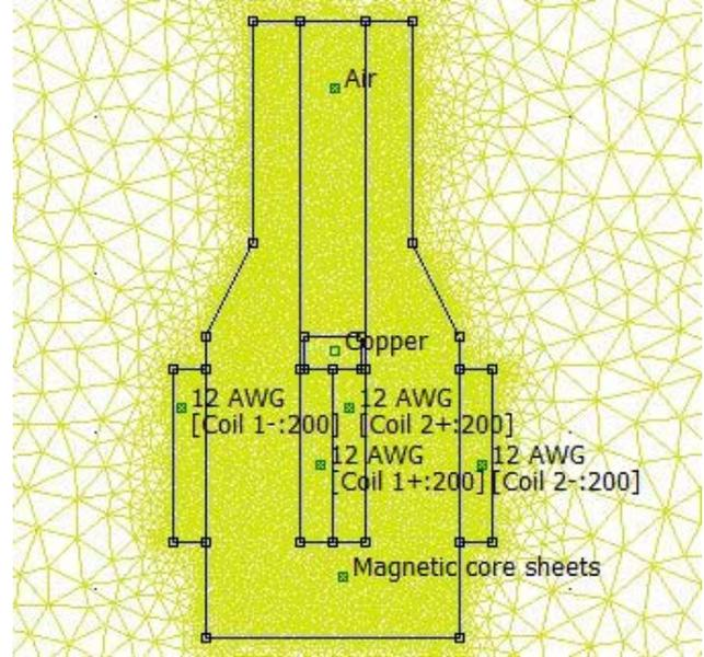
Fig. 2 – Numerical simulation of the actuator.
