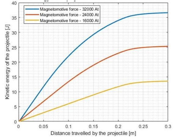
Fig. 8 – Kinetic energy as a function of trajectory / travelled distance.
