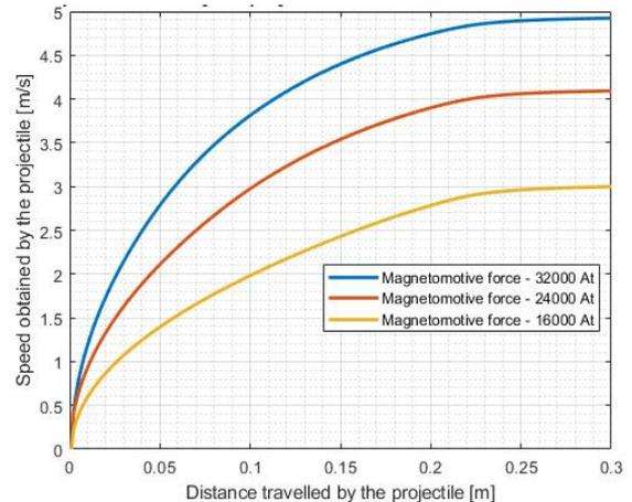
Fig. 9 – Speed as a function of trajectory / travelled distance.
