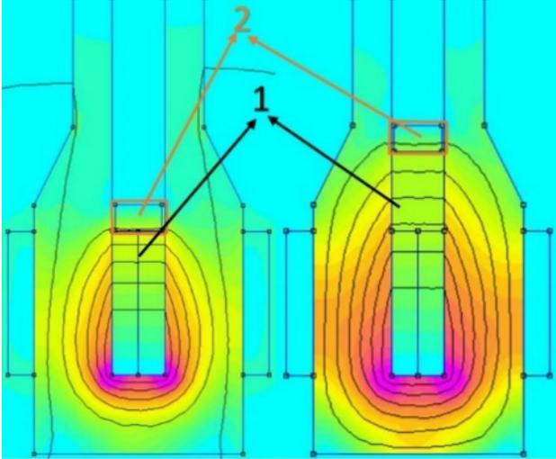
Fig. 4 – Magnetic field (1) directed by ferromagnetic circuit below the projectile (2).
