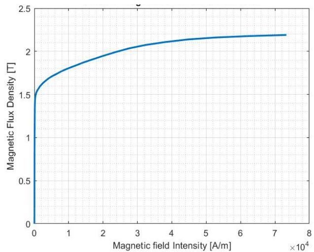
Fig. 3 – B-H characteristic of the material used for the magnetic circuit of the actuator [7].
