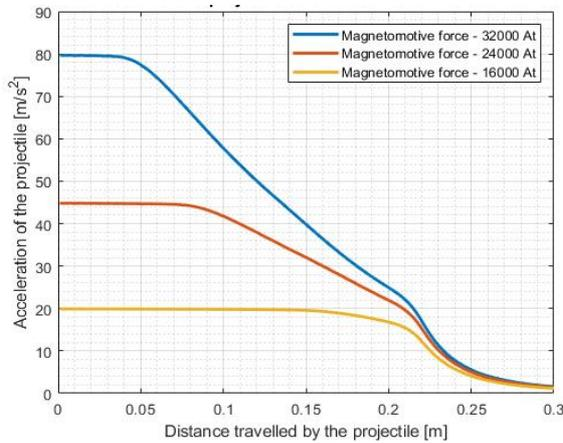
Fig. 7 – Relation between acceleration of the projectile and travelled distance.
