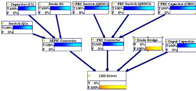
Fig. 8 – Diode bridge rectifier failure state.
