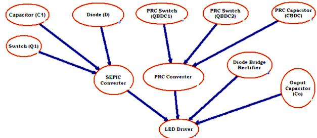
Fig. 4 – DAG representation of Bayesian structure for proposed LED driver.
