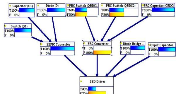
Fig. 7 – PRC Converter failure state.
