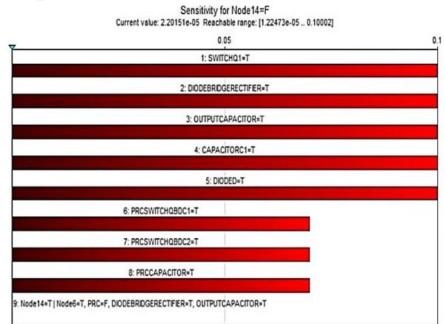
Fig. 11 – Sensitivity of LED driver using tornado diagram.
