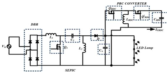
Fig. 1 – SEPIC integrated PRC LED driver.
