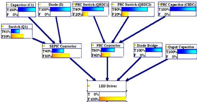
Fig. 10 – Possible failure state of LED driver.
