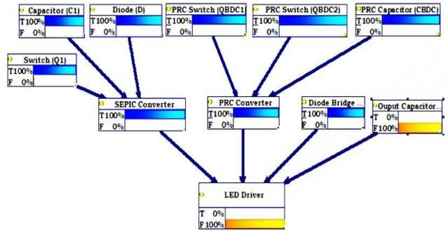
Fig. 9 – Output capacitor failure state.
