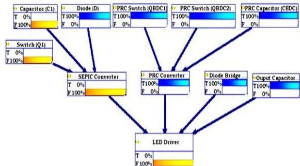
Fig. 6 – SEPIC Converter failure state.
