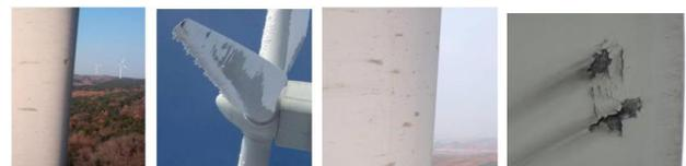
Fig. 2 – Sample images of cracked wind blade images.
