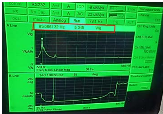
Fig. 7 – Voltage response of the piezoelectric harvester with free tip
