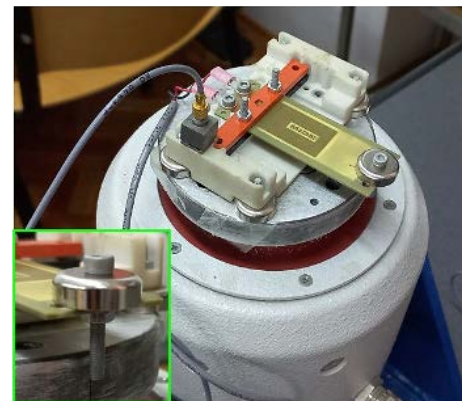
Fig. 6 – Piezoelectric harvester and detail showing tip mass mounted
