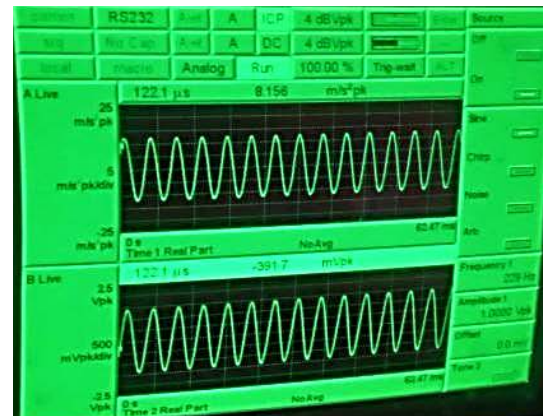
Fig. 5 –Time response of the PEH with free tip
