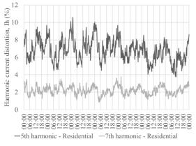
Fig. 4 – 5<sup>th</sup> and 7<sup>th</sup> harmonic current emissions as a percentage of fundamental current for configuration of residential customers in Germany [6].
