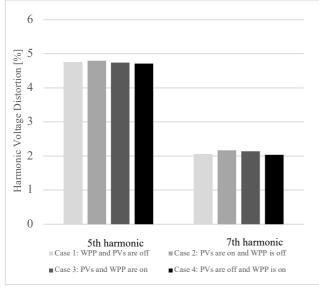
Fig. 5 – Graphical representation for four cases of harmonic voltage distortion on 0.4 kV Žabljak Usora bus.
