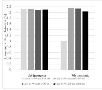
Fig. 6 – Graphical representation for four cases of harmonic voltage distortion on 0.4 kV bus Kalim.
