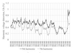
Fig. 3 – Background of the 5th and the 7th harmonic voltage distortion [6].
