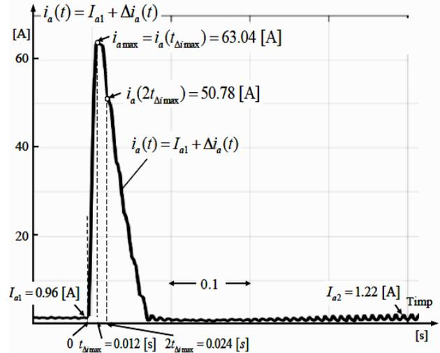
Fig. 4 – Experimental time variation (retrieved from the oscilloscope using MATLAB GUI) of the rotor-armature electrical current strength during the electromechanical transient process occurred in the sample separately-excited brushed dc motor.
