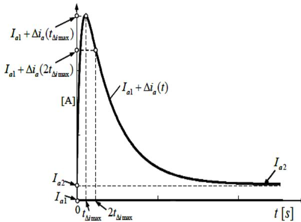
Fig. 3 – Typical time variation of the rotor-armature electrical current strength during the electromechanical transient process occurred in the separately-excited brushed dc motor.
