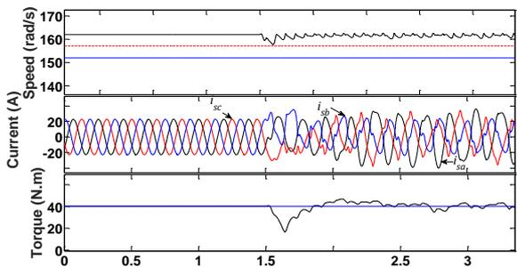
Fig. 3a<sub>1</sub> – Zoom of turn-to-turn fault effect for  $x_{sc} = 20\%$ .
