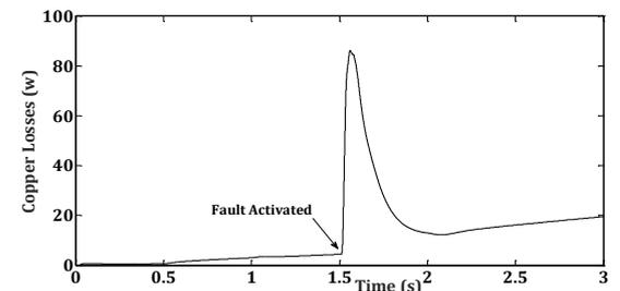
Fig. 3b<sub>2</sub> – Cooper losses evolution for  $x_{sc} = 50\%$ .
