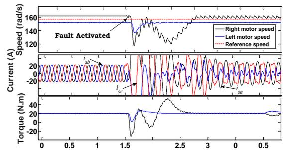
Fig. 3b<sub>1</sub> – Zoom of turn-to-turn fault effect for  $x_{sc} = 50\%$ .
