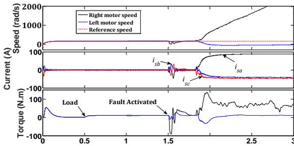
Fig. 3c – Turn-to-turn fault effect for  $x_{sc} = 100\%$ .
