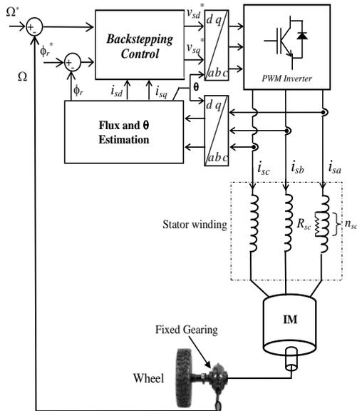
Fig. 1 – Backstepping structure of IM with turn-to-turn fault on phase *a*.
