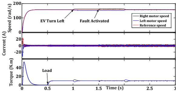
Fig. 3a – Turn-to-turn fault effect for  $x_{sc} = 20\%$ .
