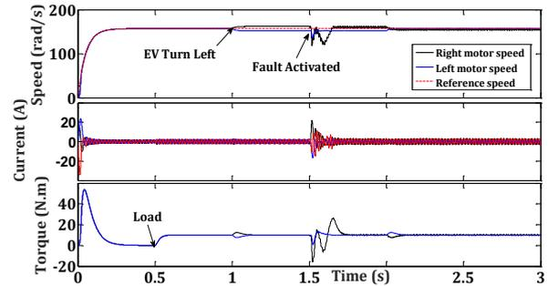
Fig. 3b – Turn-to-turn fault effect for  $x_{sc} = 50\%$ .
