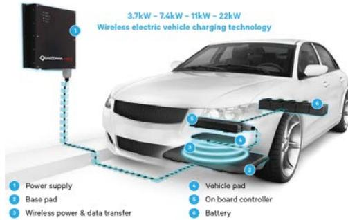
Fig. 1 – Illustrative of an inductive battery charging system by WPT, as an environmental magnetic field source [7].
