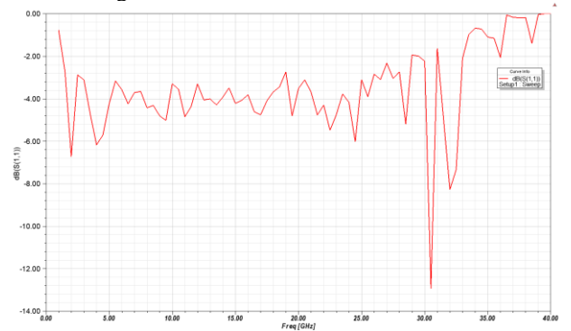
Fig. 3 – The variation of S_{11} of the slot in the frequency range 1 – 40 GHz.
