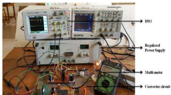
Fig. 13 – Experimental prototype of PV interfaced with proposed converter.
