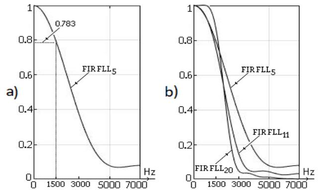
Fig. 7 – Linear magnitude of frequency responses for the half of sample rate: a. FIR FLL<sub>5</sub>, b. FIR FLL<sub>5</sub>, FIR FLL<sub>11</sub> and FIR FLL<sub>20</sub>.
