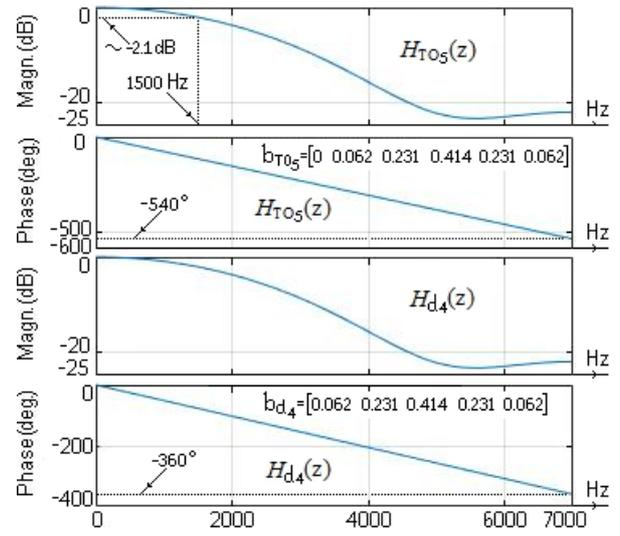
Fig. 3 – Magnitudes and phases of the frequency responses of  $H_{T05}(z)$  and  $H_{d4}(z)$ .
