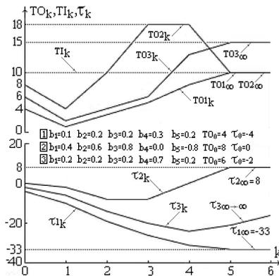
Fig. 2 – Transition and stable states of FLL<sub>5</sub> for the step input and for three cases of system parameters and the initial conditions.
