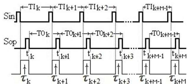
Fig. 1 – The time relations between the input and output variables of the M-th order FLL.
