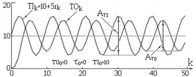
Fig. 6 – The output  $TO_k$  preserved the form of  $TI_k$ . Relation  $A_{TO}/A_{TI} = 0.776$  is very close to  $TO_{f1500}/TI_{f1500} = 0.788$ .
