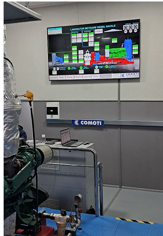
Fig. 10 – Wall display replicating the screen on the panel PC.
