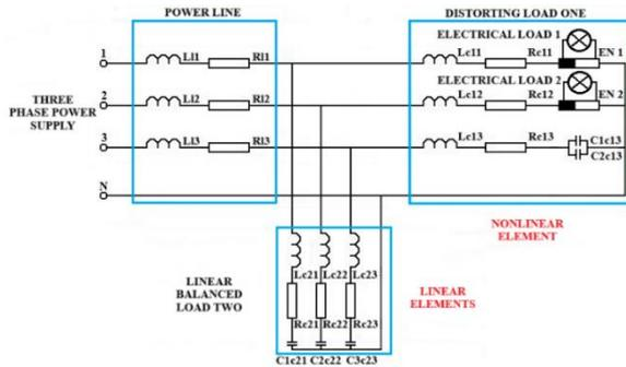
Fig. 1 – Detailed description of the experimental electrical circuit.
