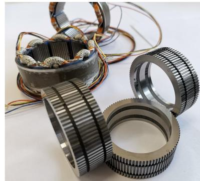
Fig. 8 – Two laminated stators and three solid rotors were manufactured.
