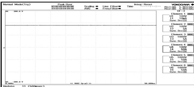
Fig. 15 – Input C voltage (rectifier output) to the Z-source network.
