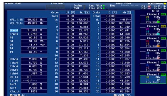
Fig. 20 – Trans-QZSI output voltage THD waveform (2.093%).
