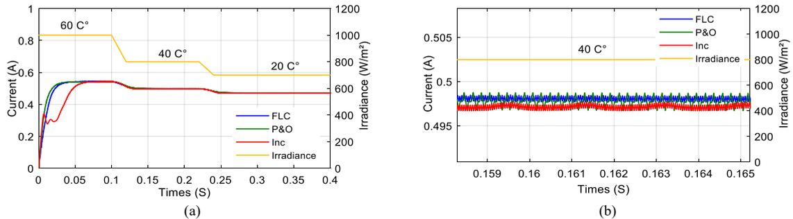
Fig. 10 – Output currents obtained by different MPPT algorithms: (a) at different levels of irradiance and temperature; (b) Zoom at 800 W/m<sup>2</sup> and 40 C.
