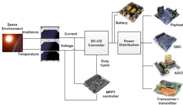
Fig. 1 – EPS based on PPT circuit.
