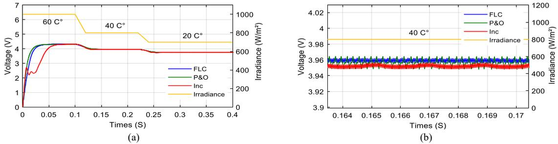
Fig. 9 – Output voltages obtained by different MPPT algorithms: (a) at different levels of irradiance and temperature; (b) Zoom at 800 W/m<sup>2</sup> and 40 C.
