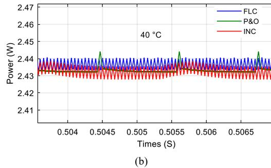
Fig. 6 – Output Powers obtained by different MPPT algorithms: (a) at different levels of temperature; (b) Zoom at 40 °C.
