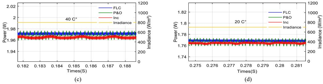
Fig. 8 – Output Powers obtained by different MPPT algorithms: (a) at different levels of irradiance and temperature; (b) Zoom at 1000 W/m<sup>2</sup>, 60°C; (c) Zoom at 800 W/m<sup>2</sup>, 40°C and (d) Zoom at 700 W/m<sup>2</sup>, 20°C.
