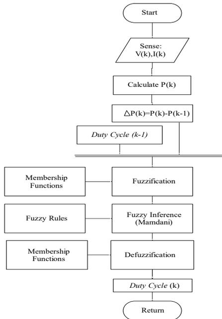
Fig. 4 – Flowchart of the proposed FLC algorithm.
