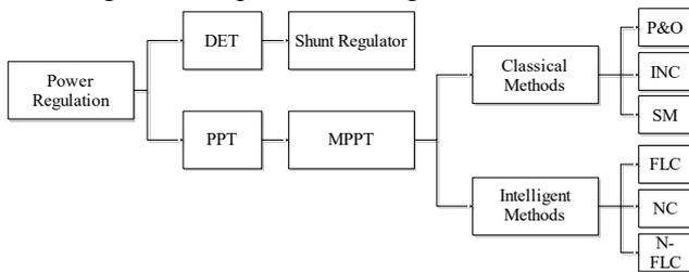
Fig. 3 – Categories of power regulation techniques based on MPPT algorithms [28].
