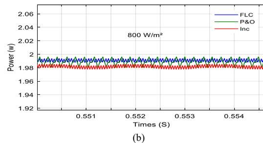
Fig. 5 – Output powers obtained by different MPPT algorithms: (a) at different levels of irradiance; (b) Zoom at 800 W/m<sup>2</sup>.
