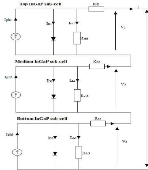
Fig. 2 – Circuit model of triple-junction solar cell.
