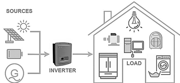
Fig. 1 – Architecture of the proposed standalone house supply system.
