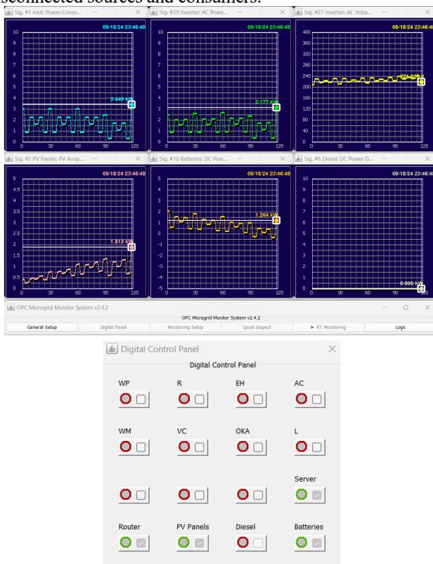
Fig. 4 – Client historical data monitoring view and digital control panel with connected/disconnected sources and consumers.
