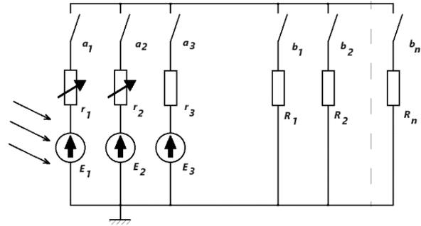
Fig. 2 – Equivalent electric circuit with three sources and  $N$  consumers.
