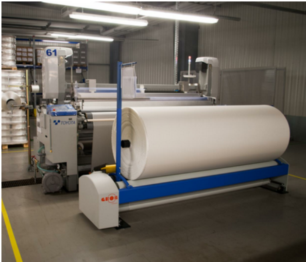
Fig. 1 – The Toyota water jet loom used for airbag fabric.
