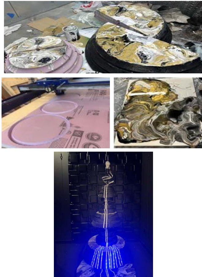
Fig. 2 – A CNC machine to carve foam into bowl shapes and used paint-pouring techniques to create marbling textures. The final sculpture displays LED lights that repeat continuously in the Wilkinson building at Duke University.
