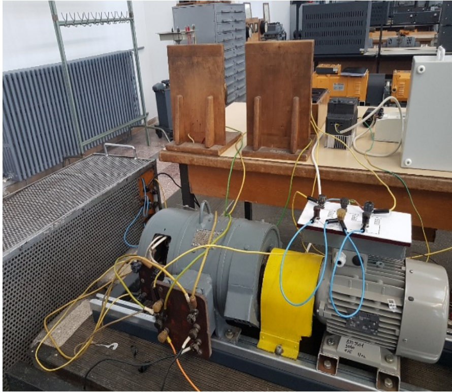
Fig. 4. Physical platform for induction motor – machines side
